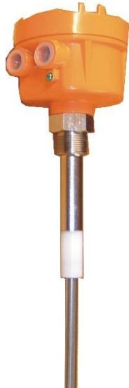
Much like radar, capacitance is based on the dielectric of the product. It is a versatile technology and provides simple, accurate and reliable level control for a wide range of applications. Capacitance is suitable for use on liquids, solids, slurries, pastes, granules, powders and pellets, and operates in high-temperature, high-pressure or corrosive environments.
