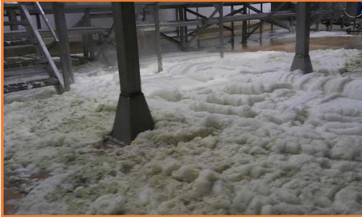
Most of the common foams are an unstable, two-phase medium of gas and liquid with a particular structure consisting of gas pockets trapped in a network of thin liquid films and plateau borders. Several conditions are needed to produce foam: there must be aeration (generated for example by mechanical agitation, mixing, stirring and sparging)
